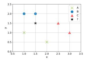
Figure 1: k-NN example: To classify the given *test* point  $\star$ , we simply assign it the majority label of the k nearest *training* points. For example, the k = 3 nearest neighbors have class labels A, B, B, so we label the new point as B.
