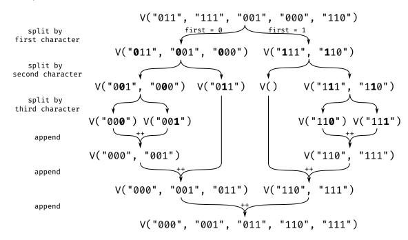
Since the sorting for bitstrings starting with 0 and those starting with 1 are independent, we can parallelize them. Below we show an implementation of a parallel radix sort for bitstrings.
